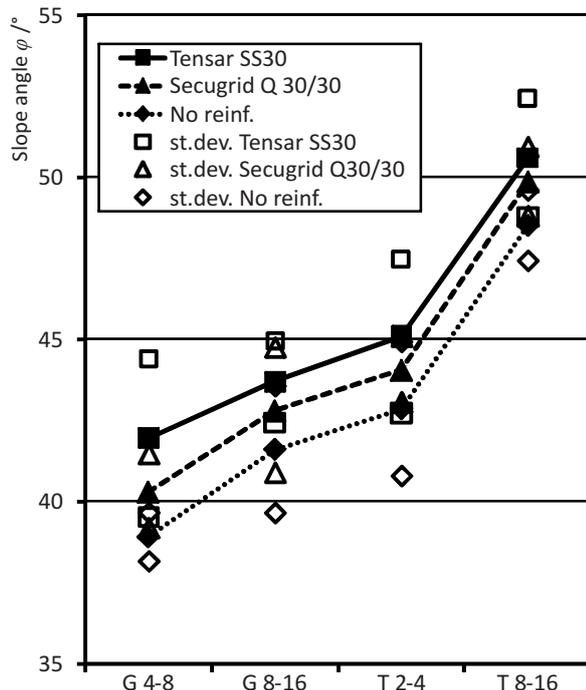
**Figure 8** Mean values of slope angles with test standard deviations for nonreinforced soil and for soil reinforced with geogrids Tensar SS30 and Secugrid Q30/30 in natural gravel G 4-8, G 8-16 and crushed gravel T 2-4 and T8-16.
