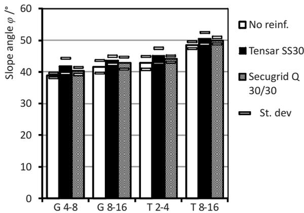
**Figure 7** Mean values of natural slope angles with tests standard deviations measured for soil alone, geogrids Tensar SS30 and Secugrid Q30/30 in natural gravel G 4-8, G 8-16 and crushed gravel T 2-4 and T8-16.
