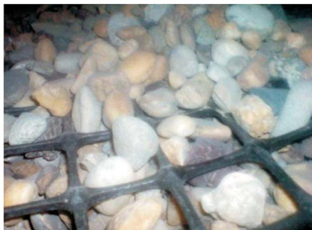
Figure 3 Grid and gravel particles arrangement in reinforced soil
