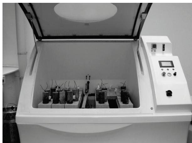
**Figure 2** Specimens exposed to simulated marine environment in salt spray chamber
