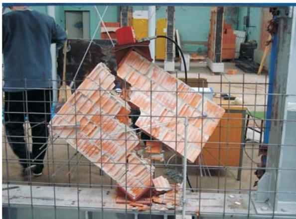
Figure 12 Total separation of the test sample
