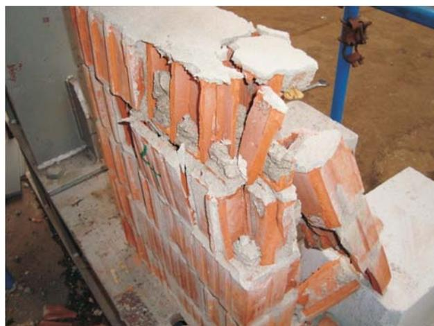
Figure 3. The test sample after failure in compression
