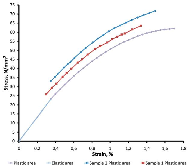
Figure 10 Comparison of different  $\sigma$ - $\epsilon$  diagrams
