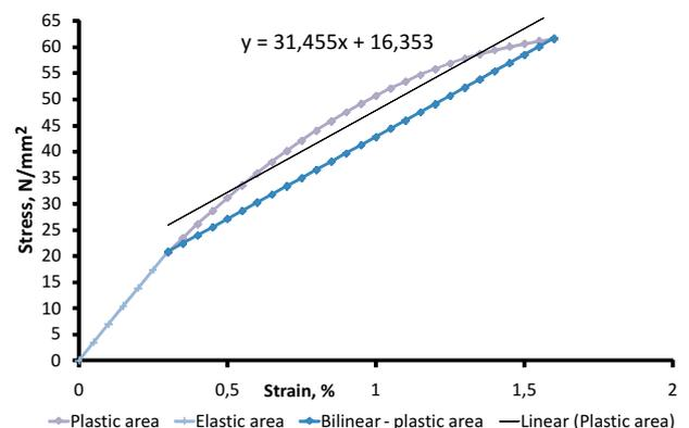
Figure 9 Idealised bilinear  $\sigma$ - $\varepsilon$  diagram
