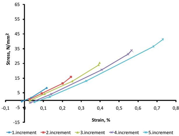
Figure 6  $\sigma$ - $\varepsilon$  diagram, sample 2, 5 increments, releasing stress
