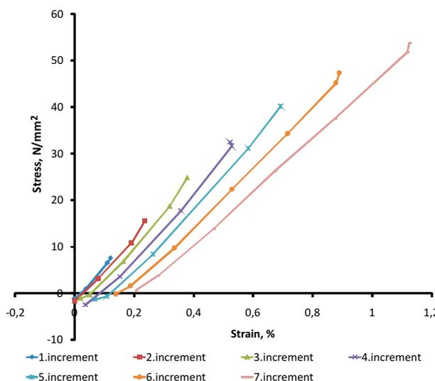
Figure 4  $\sigma$ - $\epsilon$  diagram, sample 1, 7 increments, releasing stress
