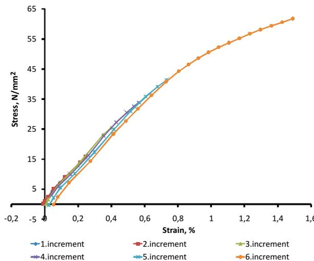
Figure 5  $\sigma$ - $\epsilon$  diagram, sample 2, 6 increments, applying stress
