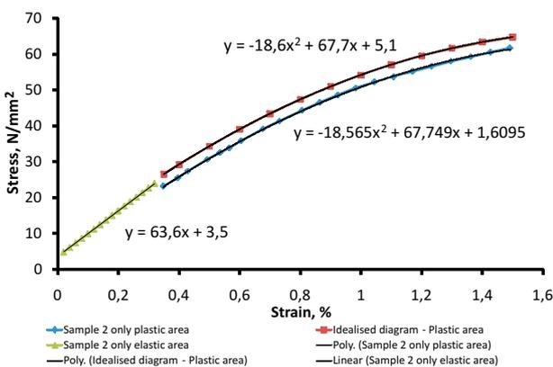
Figure 8 Idealised  $\sigma$ - $\varepsilon$  diagram – sample 2
