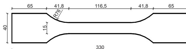
**Figure 1** Geometry of the tested GFRP sample (units in mm)
