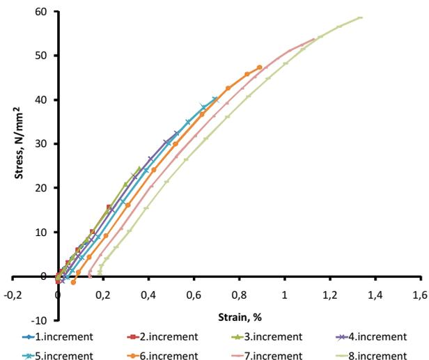
Figure 3  $\sigma$ - $\epsilon$  diagram, sample 1, 8 increments, applying stress
