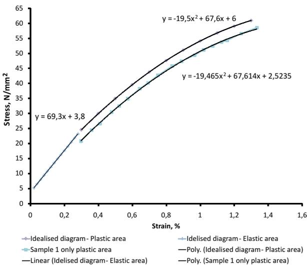
Figure 7 Idealised  $\sigma$ - $\varepsilon$  diagram – sample 1
