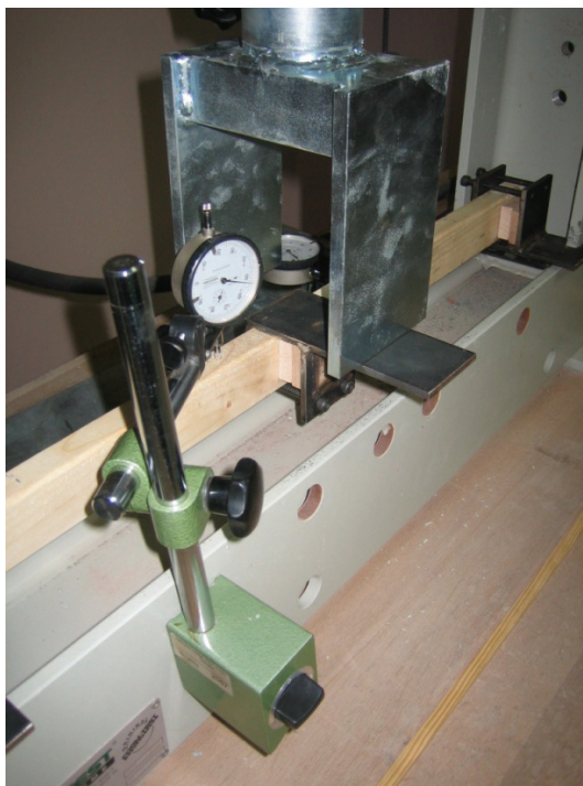
Figure 4 Measuring of deformation and applying of load
