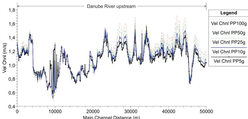
Figure 9 Distribution of velocities in the longitudinal section of the Danube River upstream from the Drava mouth
