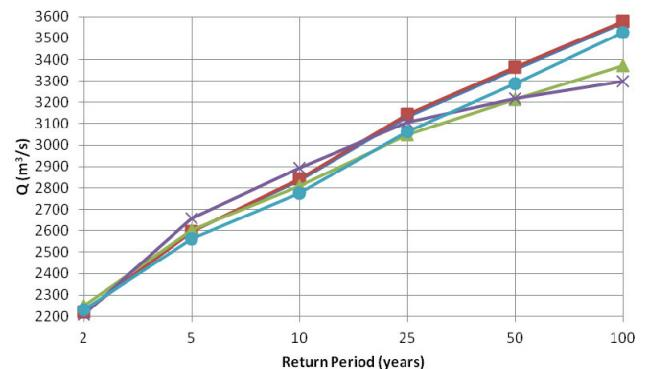
Figure 6 Values of the Danube River discharges obtained by different distributions
