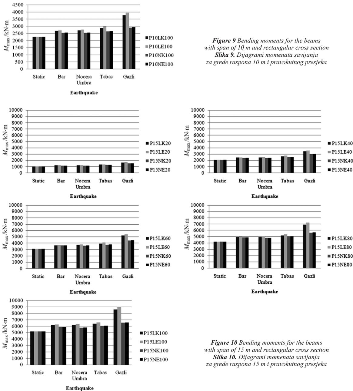
Figure 10 Bending moments for the beams with span of 15 m and rectangular cross section
