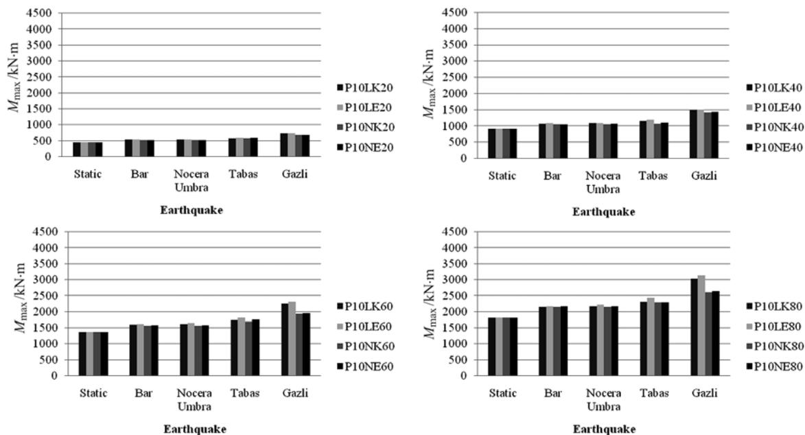
Figure 9 Bending moments for the beams with span of 10 m and rectangular cross section
