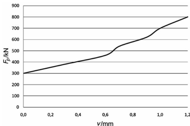
**Figure 4** Force-deflection diagram of the elastomeric bearing test [10]
