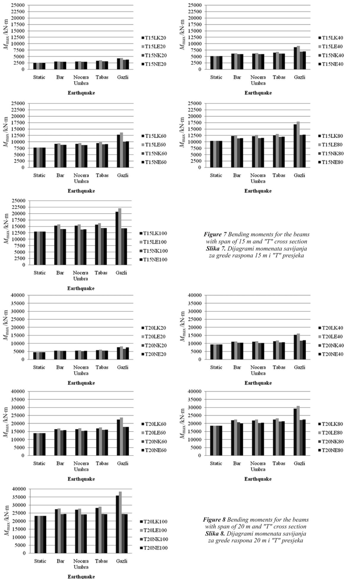
Figure 7 Bending moments for the beams with span of 15 m and "T" cross section
