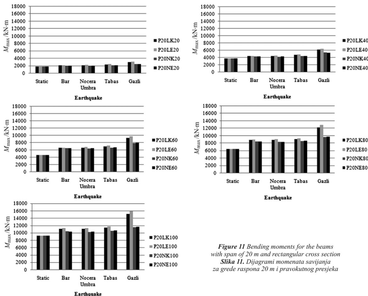
Figure 11 Bending moments for the beams with span of 20 m and rectangular cross section
