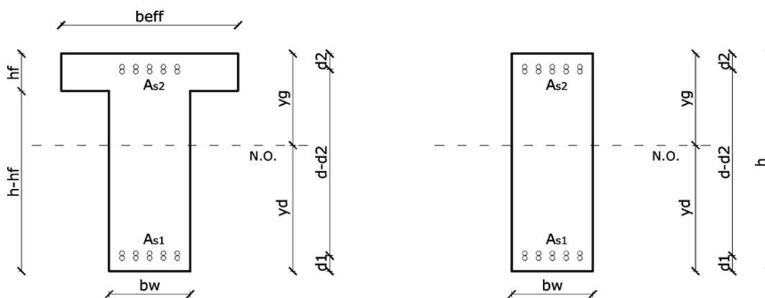
Figure 5 Cross sections of the beams
