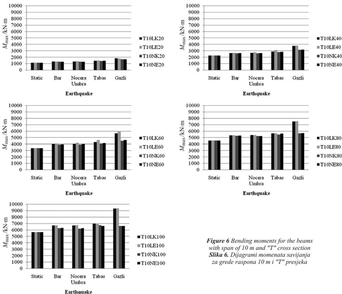
**Figure 6** Bending moments for the beams with span of 10 m and "T" cross section
