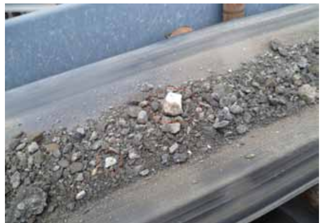
Figure 7. Recycled asphalt obtained by milling the bituminized base course
