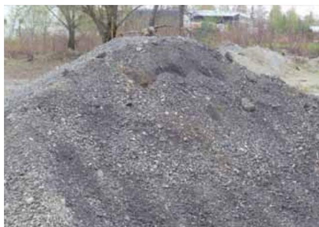
Figure 1. Recycled asphalt stockpile
