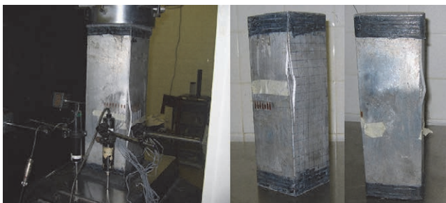
Figure 6. Testing (left) and failure mode (right) of hollow square aluminium sections filled with concrete [37]
