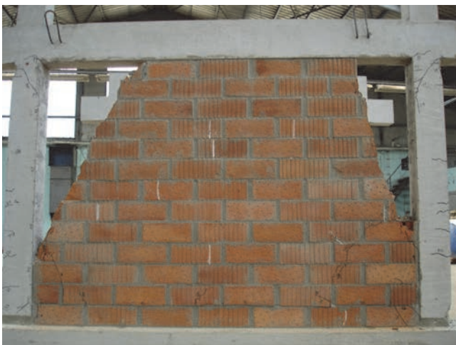
Figure 6. Failure of masonry infill walls made with hollow clay units (specimens O1_{bpm} and O3_{bpm} )
