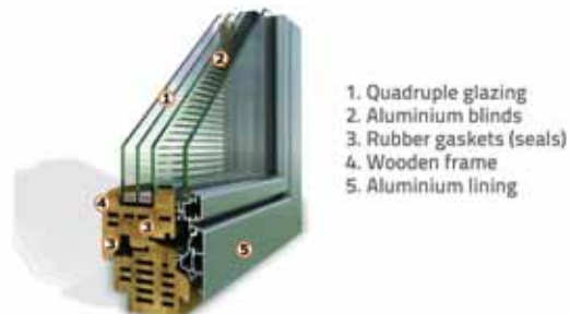
Figure 16. Wooden window with quadruple glazing
