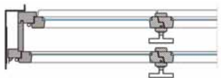
Figure 10. Horizontal cross-section of double double-sash window
