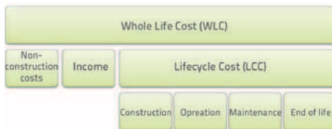
Figure 1. Whole life cycle cost and life cycle cost structure [16]
