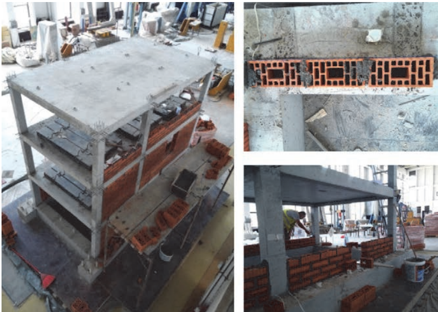
Figure 1. Clay block masonry infill construction as per [4]
