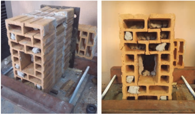
Figure 6. Clay block tensile failure due to masonry bond with interlocking
