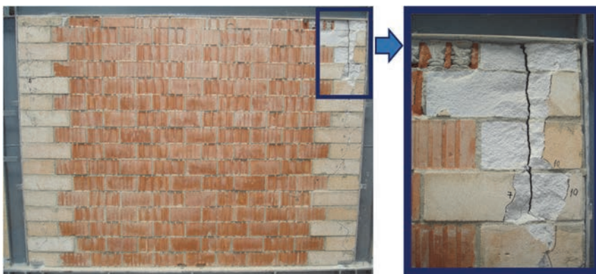
Figure 6. Photographs of specimen CA-1 after failure
