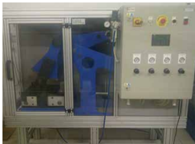
Figure 3. Roller compactor for compacting asphalt course in the mould
