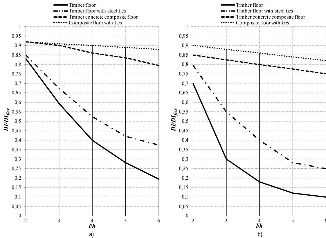
Figure 2 Diagram relating  $(DI/DI_{RC})$  to  $(l/h)$  for URM buildings up to three storeys and a)  $0.15 < f_t < 0.25$  MPa [22] b)  $f_t < 0.15$  MPa [22]
