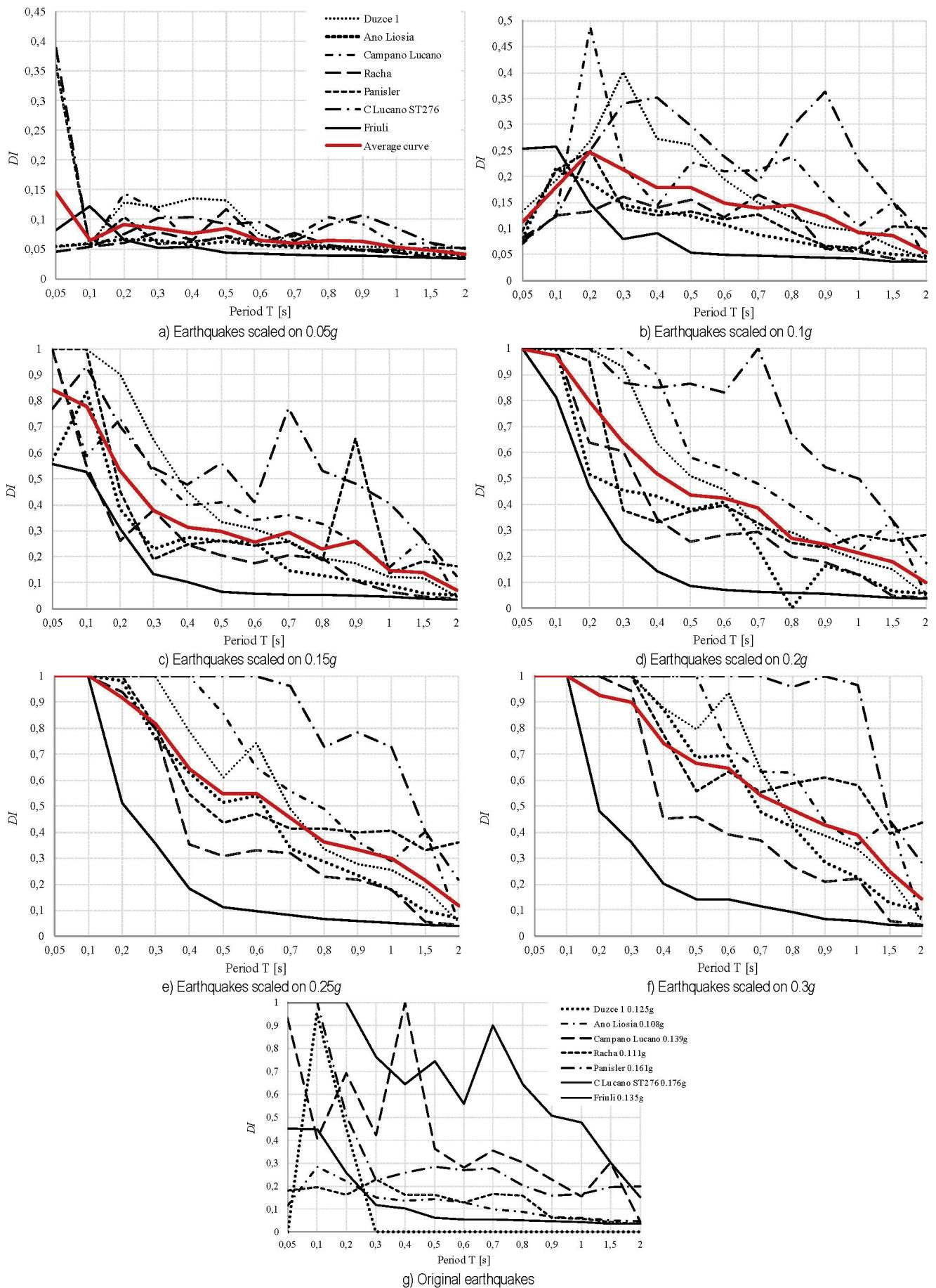
Figure 4 Spectral damage functions for URM with flexible floors defined by the following parameters  $BS_1=0.1$ ,  $WK_2=0K_0$ ,  $\zeta=5\%$  and a) earthquakes: scaled on 0.05g, b) Earthquakes scaled on 0.1g, c) Earthquakes scaled on 0.15g, d) Earthquakes scaled on 0.2g, e) Earthquakes scaled on 0.25g, f) Earthquakes scaled on 0.3g, g) Original earthquakes
