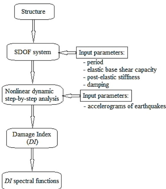
Figure 1 Proposed methodology for seismic vulnerability assessment
