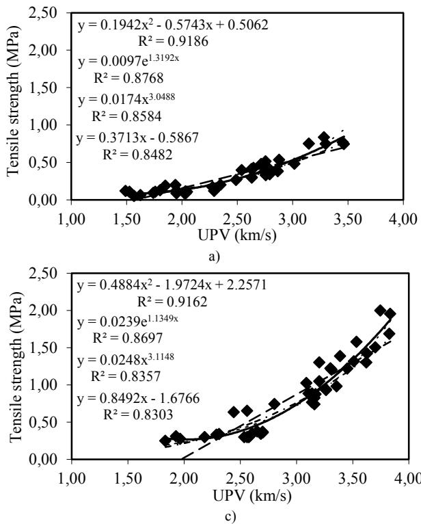
Figure 7 Relation between pulse velocity and indirect tensile strength for a) 7; b) 28 and c) 90 days curing period
