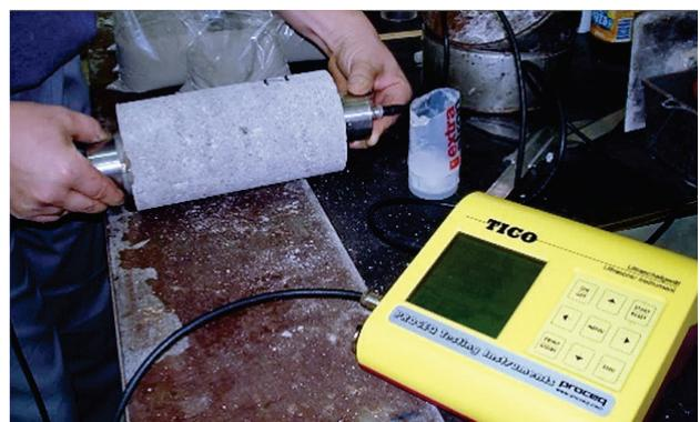
**Figure 2** Measurement of ultrasound pulse velocity
