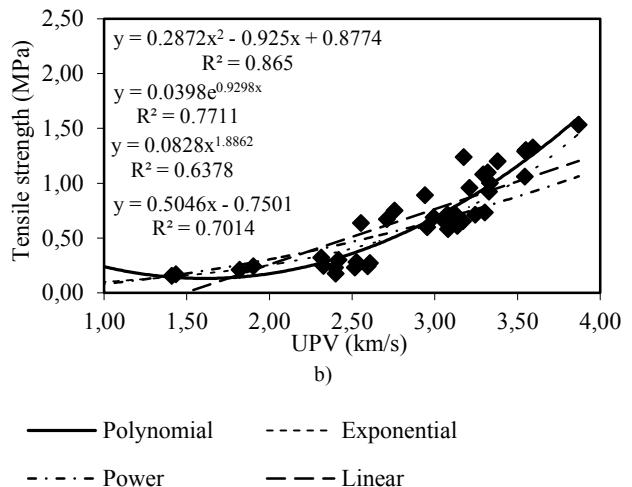
Fig. 5b can be seen that for this range of compressive strength, characteristic UPV values can be determined. For UPV less than 2 km/s and more than 3,2 km/s, cement stabilized material can be classified as inappropriate for road construction purposes since it has compressive strength less than 2 MPa i.e. more than 6 MPa. For UPV values between 2 and 3,2 km/s, cement stabilized material can be classified as good quality material for road construction purposes.
